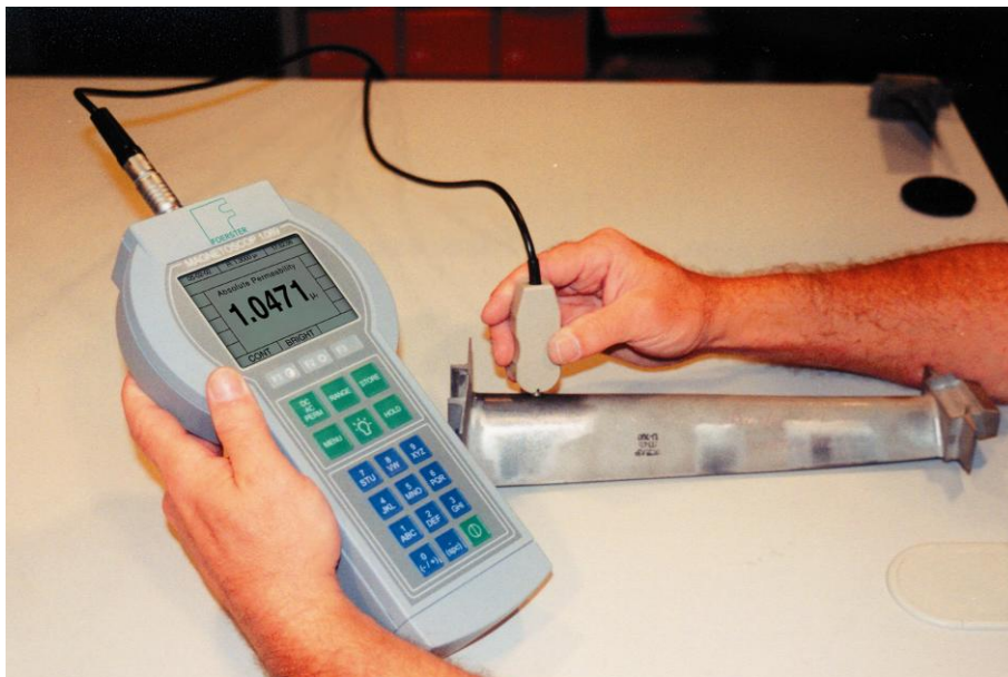
Figure 2 MAGNETOSCOP 1.069, Permeability measurement on a turbineblade with permeability probe
